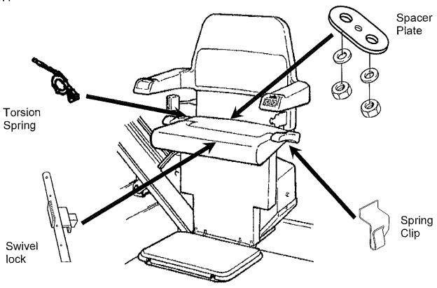
The swivel seat can fail to safely lock in position under extreme circumstance of abuse or excessive use. This is due to wear of the swivel lock assembly and has occurred in a few instances with stairlifts permanently in use since 1995.
