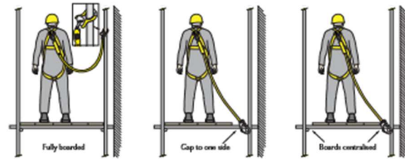
Figure 14: Fully boarded platform with a maximum of one board gap (225mm) may be permitted only if required to access the ledge below the platform as an anchor point.
