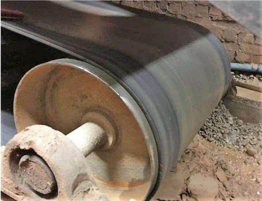
*Entanglement in conveyor systems is a significant cause of serious incidents in the quarry industry. Quarry operators should make sure they properly assess and apply effective control measures to minimise the risk from dangerous parts of machiner. "*
