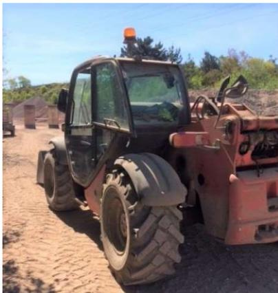
*"The director was aware of the unsafe condition of the telehandler yet allowed it to be used by an inexperienced employee. HSE promotes safe-stop procedures where drivers should apply the parking brake and turn off the ignition before exiting any mobile machinery. This could not be done as the telehandler was in such poor mechanical condition. Maintenance is not optional. This accident could easily have been prevented."*
