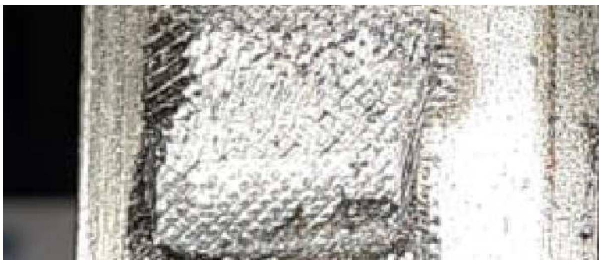
INCORRECT mark, knurling not well marked and with hollow on the rail.
